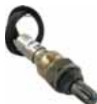
XOS00413. Oxygen sensor. Suits Universal Applications 4 wire 13 \Omega . Measures and determines unburnt oxygen content in the exhaust gas and reports to the ECU.
