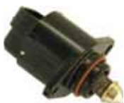
XIS10011. Idle speed control. Suits Holden Camira, Astra, Frontera 1.8, 2.0, 2.2. Controls the idle speed of the vehicle by altering airflow.
