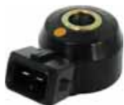
XKS1007. Knock sensor. Suits Nissan. Fitted to the engine block to detect detonation and other abnormal engine vibrations sending messages to the ECU.
