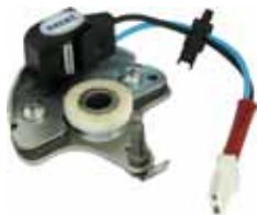
PUC150148. Pick-up coil. Suits Fiat Regatta, Ritmo, Tempna, Tipo, Uno. In-distributor pick-up coils send small amount of volts to the vehicle's ignition module.
