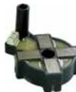
XIC5107. In-distributor coil. Suits Ford Telstar, Ford Laser, Mazda 323 and 626 -.
