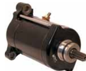
STR11416. ATV starter motor. Suits Honda Foreman TRX400, 450, 500.
